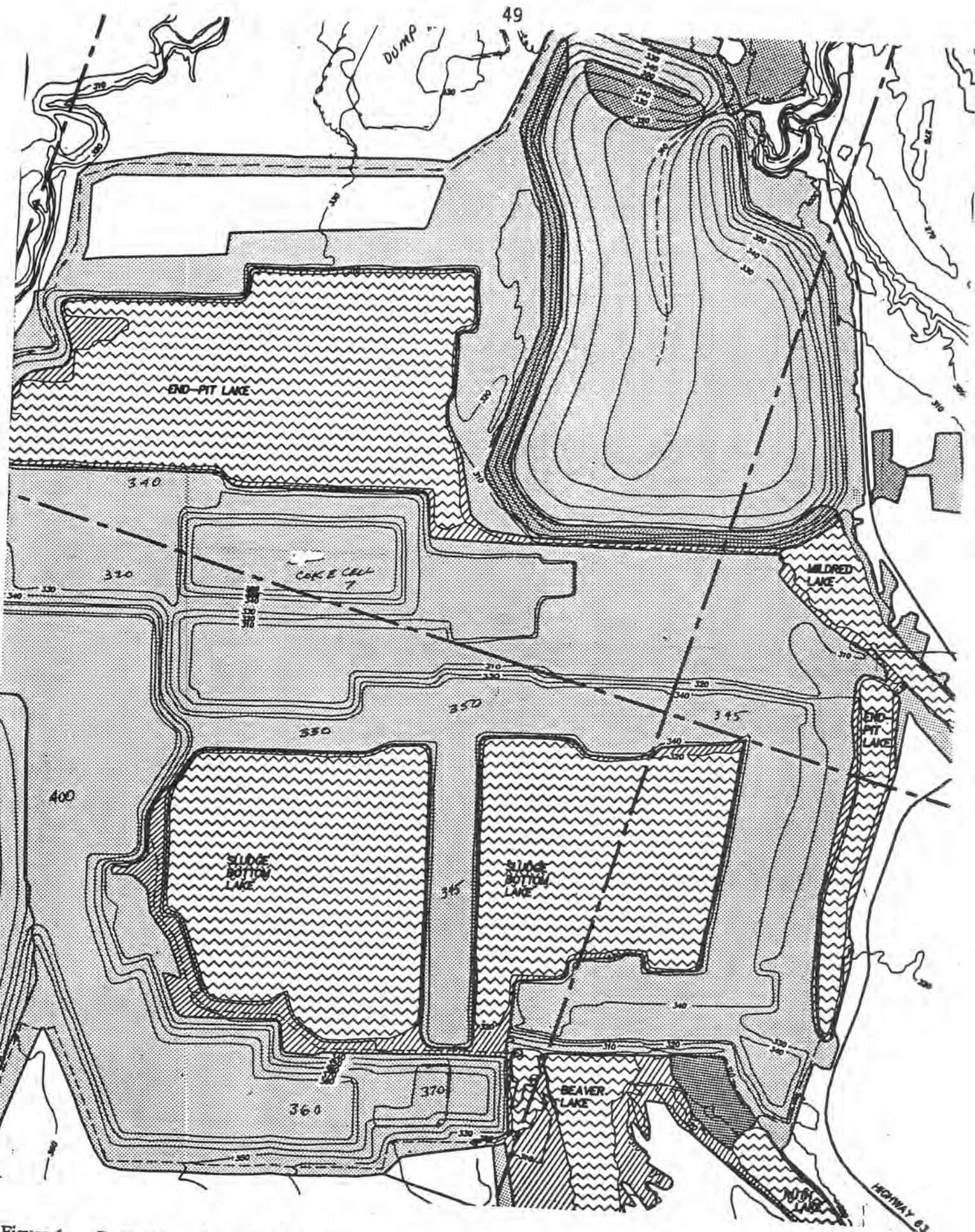
Figure 1: Proposed configuration of fines-bottom lakes as described in Syncrude's 1988 Development and Reclamation Plan.
